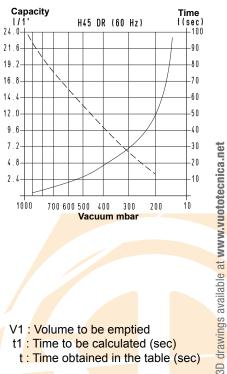
To calculate the emptying time of a volume V1, apply the formula  $t_{1} = \frac{t_{X}V_{1}}{6}$
